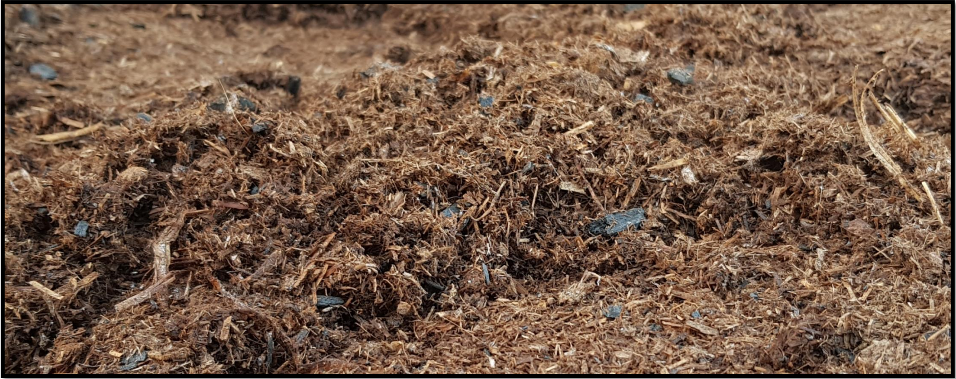
Figure 2: COM-BI blend at 19.8 % w/w d.b. of biochar content
